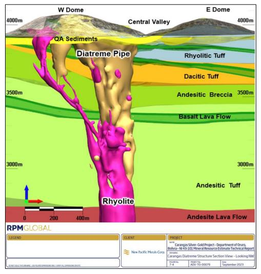
Figure 7-4 Carangas diatreme structure section view – looking NW
