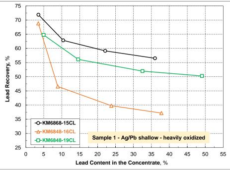
Figure 13-6 Lead recovery and lead content in the concentrate for Sample 1
