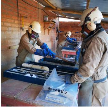
Figure 11-2 Core cutting and sample bag
