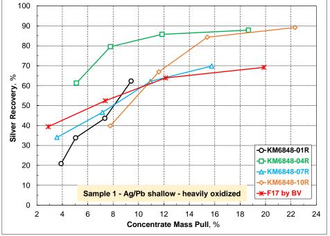
Figure 13-3 Silver recovery as a function of concentrate mass pull for Sample 1 by ALS
