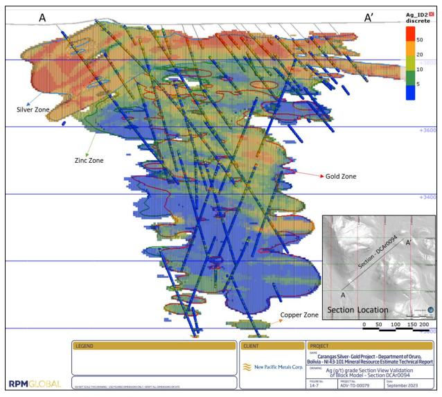
Figure 14-7 Ag (g/t) grade Section View Validation of Block Model – Section DCAr0094
