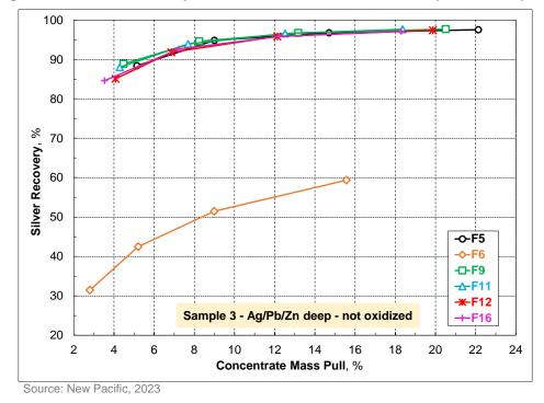
Figure 13-15 Silver recovery as a function of concentrate mass pull for Sample 3
