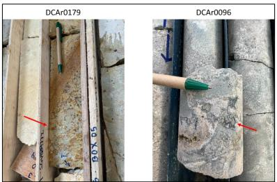
Figure 12-1 Drill core mineralization intercepts examples
