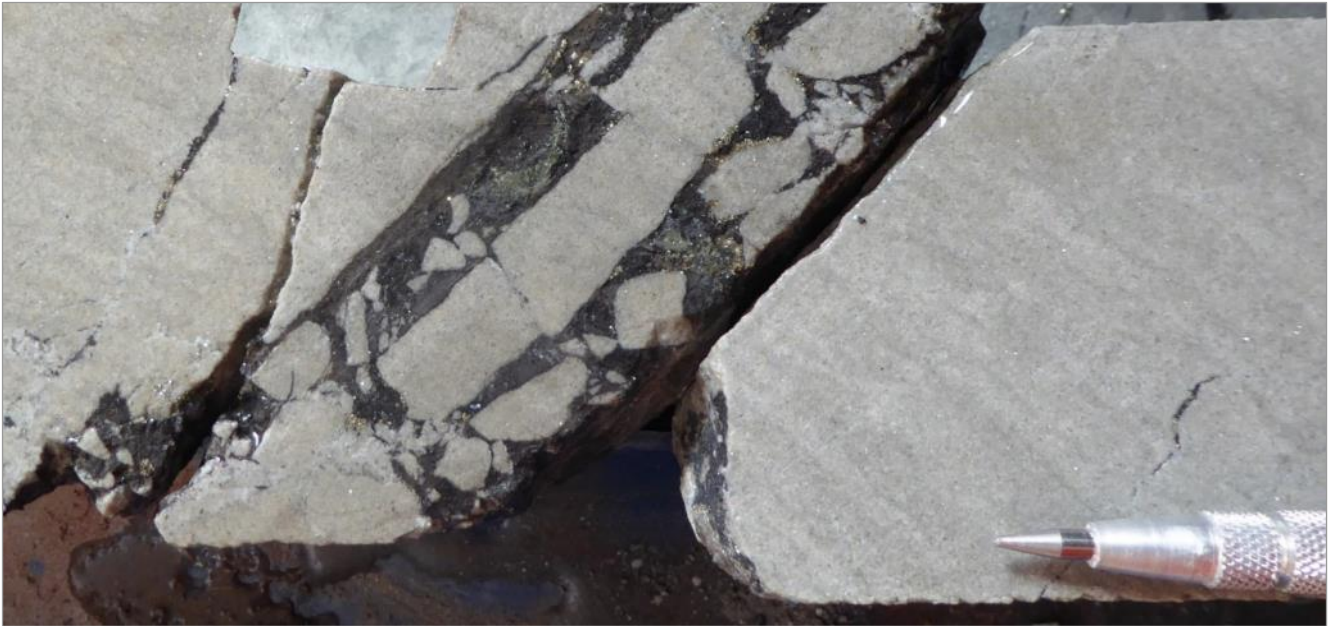
Note: DSS565001 Sulphides and sulfosalts crackle breccia @ 141 m (265 g/t Ag, 0.28% Pb, 1.51% Zn). Source: New Pacific Metals Corp., 2019.
