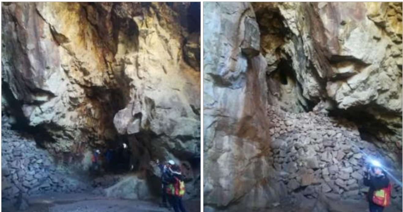
Figure 9.5 Mineralized structures and fractures in historically mined Snake zone glory hole
