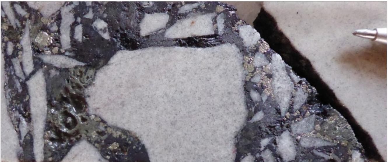
Note: DSS665001 Sulphides and sulfosalts crackle breccia @ 125.81 m (1,290 g/t Ag, 0.92% Pb, 4.05% Zn). Source: New Pacific Metals Corp., 2019.
