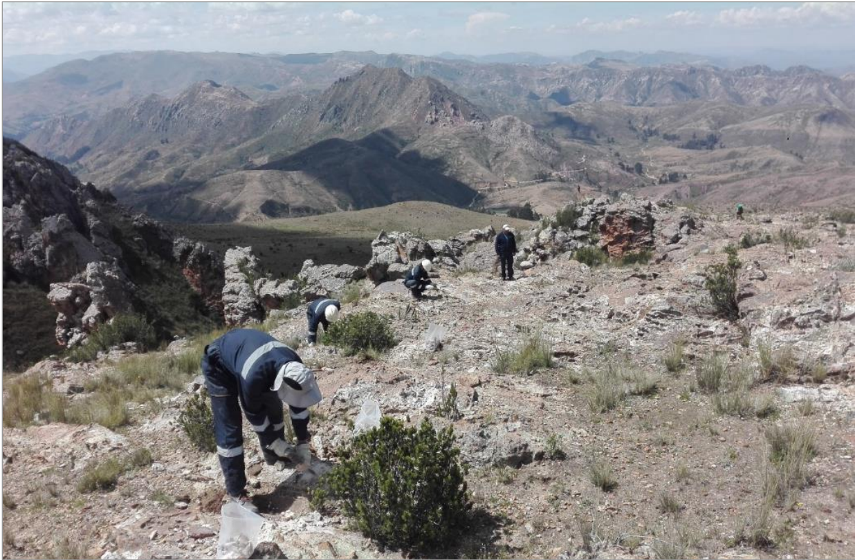
Figure 9.3 Channel sampling at the Jordan Prospect
