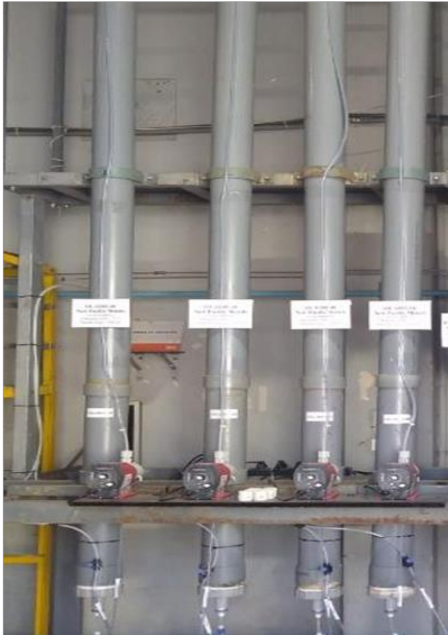
Figure 13.3 Column leaching test setup
